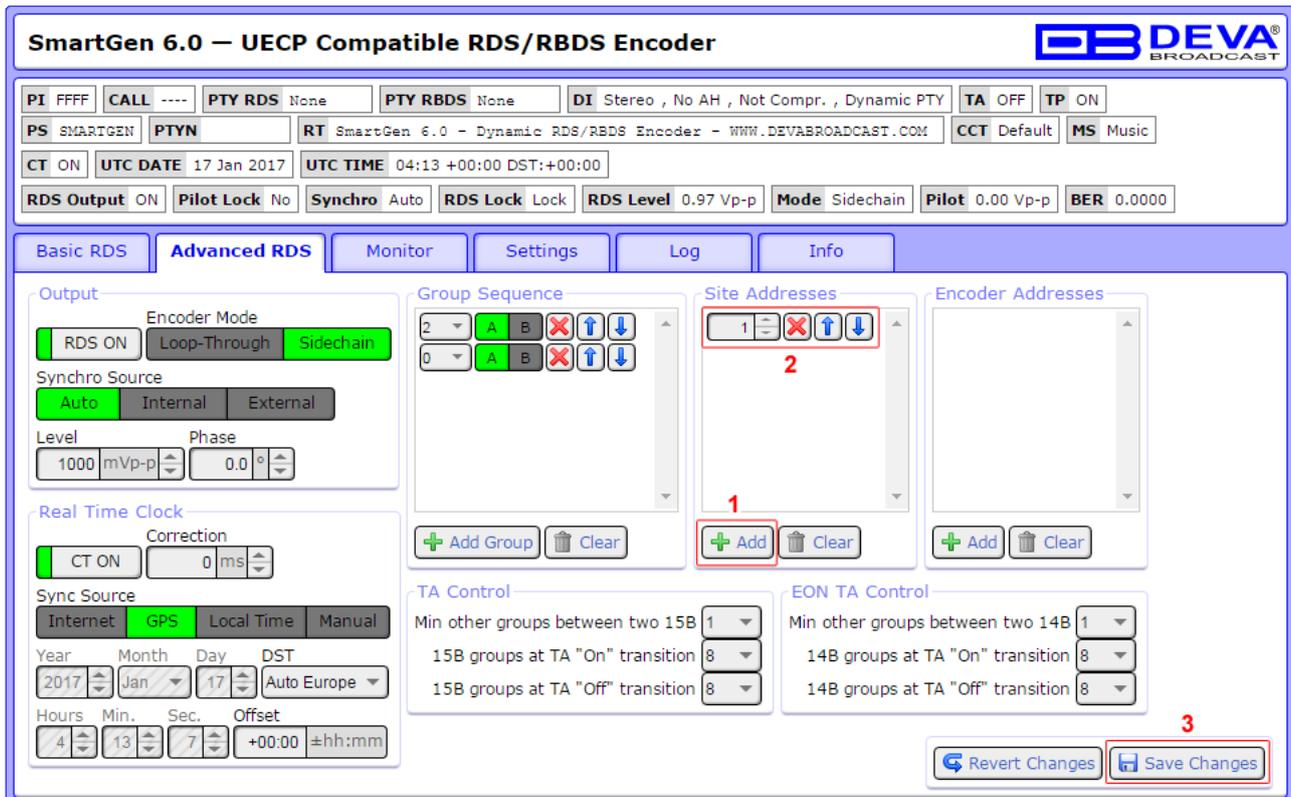
The screenshot shows the 'Advanced RDS' configuration page. The 'Site Addresses' section contains a list with one entry '1'. A red box labeled '1' highlights the '+ Add' button below the list. A second red box labeled '2' highlights the '1' in the list. A third red box labeled '3' highlights the 'Save Changes' button at the bottom right of the interface.
