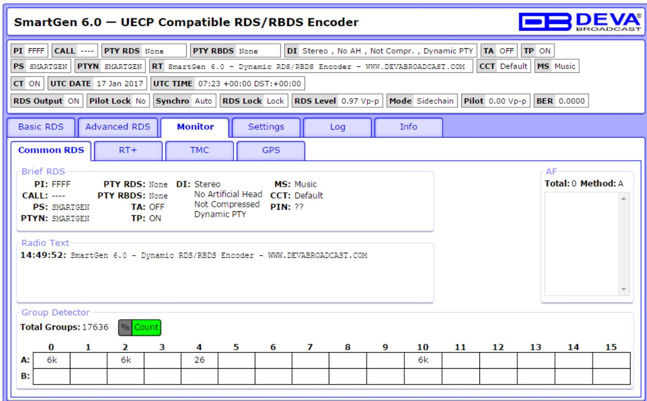
The screenshot shows the 'Monitor' tab of the 'SmartGen 6.0 – UECP Compatible RDS/RBDS Encoder' interface. The 'Common RDS' section is active, displaying the following parameters:
