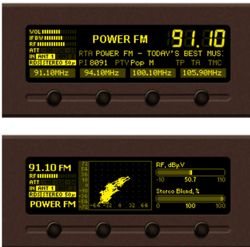
OLED display with function areas
