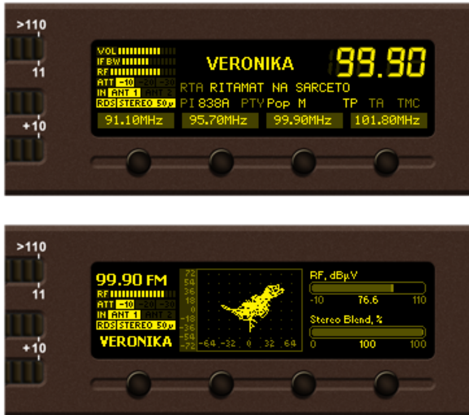
OLED Display with its function areas
